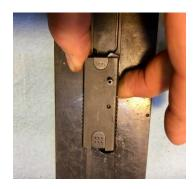
Start extractor roll pin into top of slide. Insert extractor spring and extractor into slide and hold flush to side of slide. Make sure extractor is pulled back onto the breech block face. This will create proper alignment for the roll pin. Drive extractor roll pin just past flush using a 1/8" roll pin punch.
