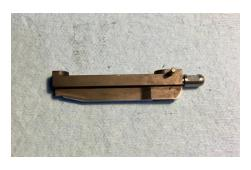
Start the firing pin retaining pin into the breech block. Install the firing pin and firing pin spring. Index the firing pin head notch so as the retaining pin goes in it clears the firing pin without damage. Set on a hard surface and compress the breech block assembly while driving the retaining pin to flush.
