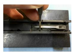
Use a small roll pin punch and remove the extractor roll pin. This MUST be driven from bottom through top or damage to the slide will occur. Remove extractor and spring from slide and set aside.
